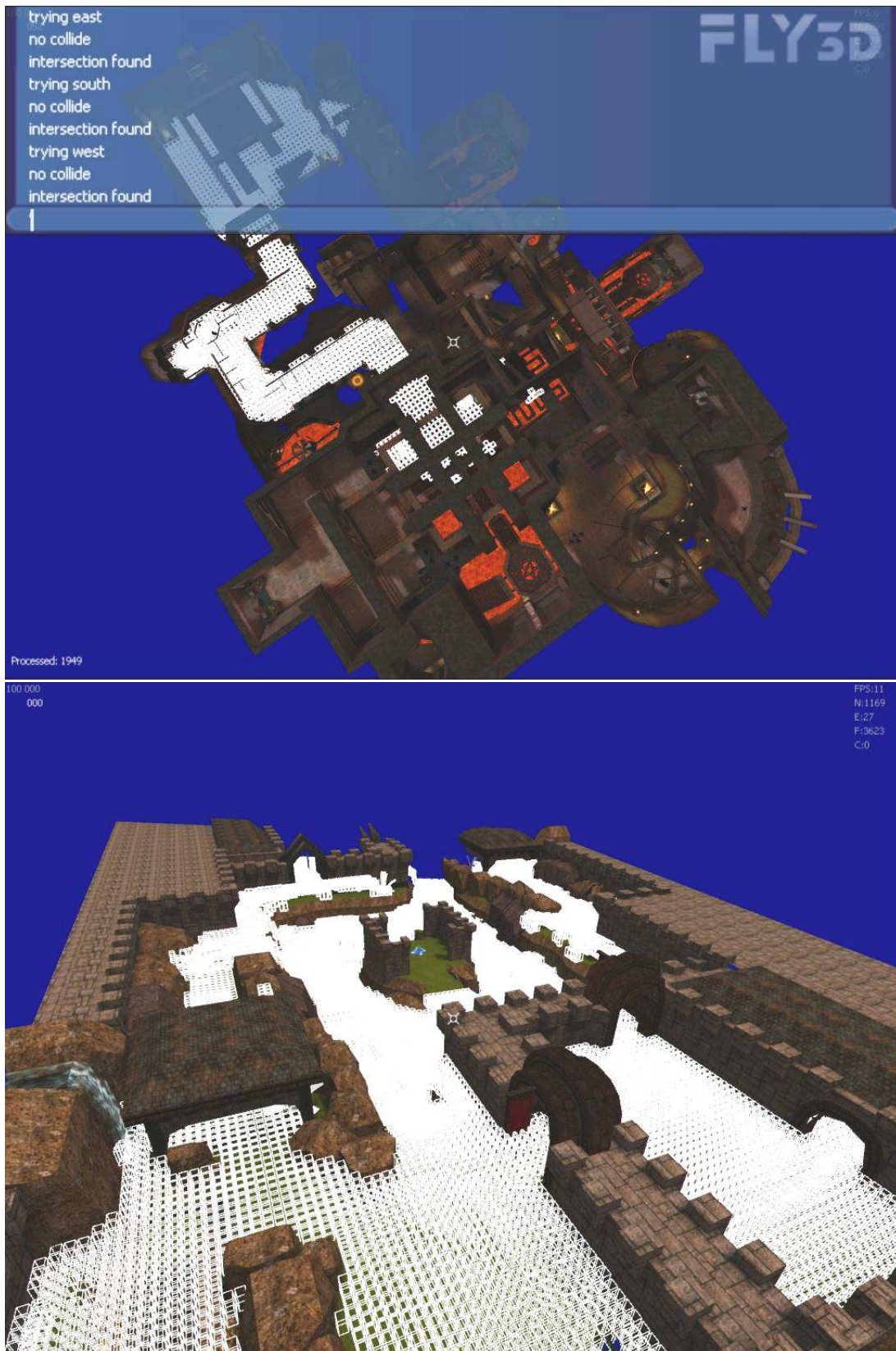
Figure 4.3: Above - partially generated stage one area awareness data for a very complex environment. Below - stage one area awareness data for the environment used in the second implementation.
