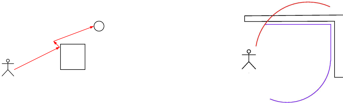
Figure 3.9: Left - a typical example of the first obstacle avoidance technique in action, the agent encounters an obstacle on the path to a node, moves off in a random direction and continues unobstructed. Right - a typical example of the second obstacle avoidance technique, the agents original curving path, part of a strafing maneuver, is represented in red, in blue is the adjusted path to handle the obstructing wall.
