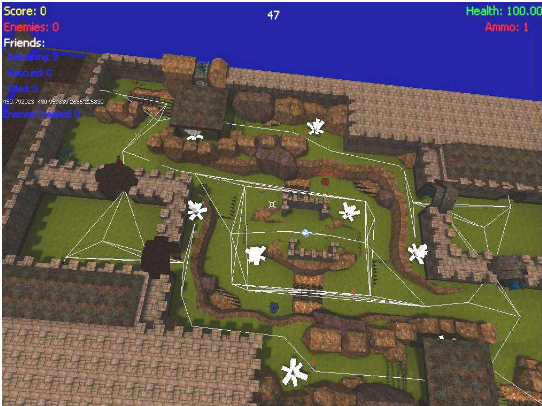
Figure 3.7: An example screenshot showing a section of a navigation node graph. The white lines overlaid on the environment are the edges of the graph, nodes are not actually drawn but are positioned at the endpoints of edges.
